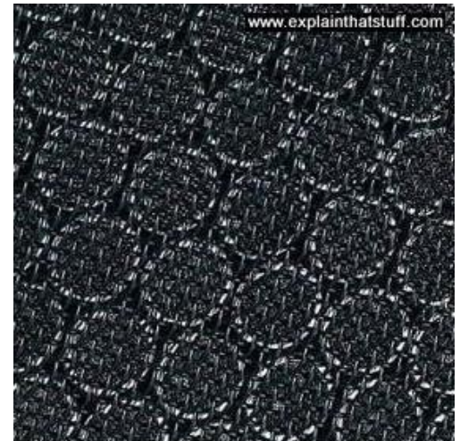
Photo: A parametric, directional speaker has an Array of many ultrasonic transducers
