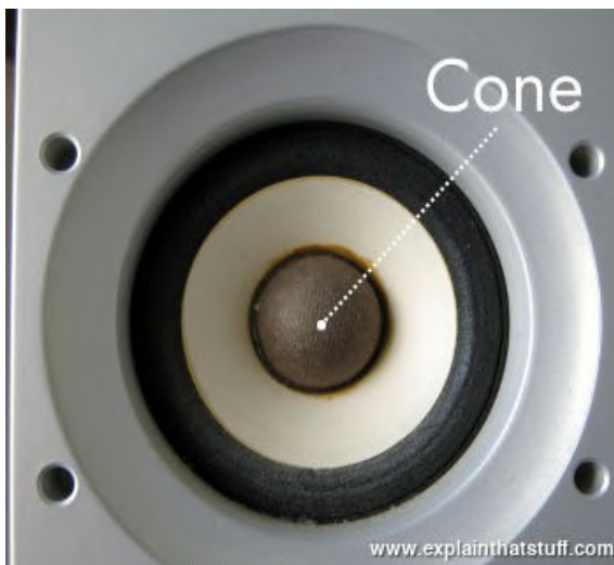
Photo: A conventional (electromagnetic) speaker Has a single, large, sound-producing cone.
